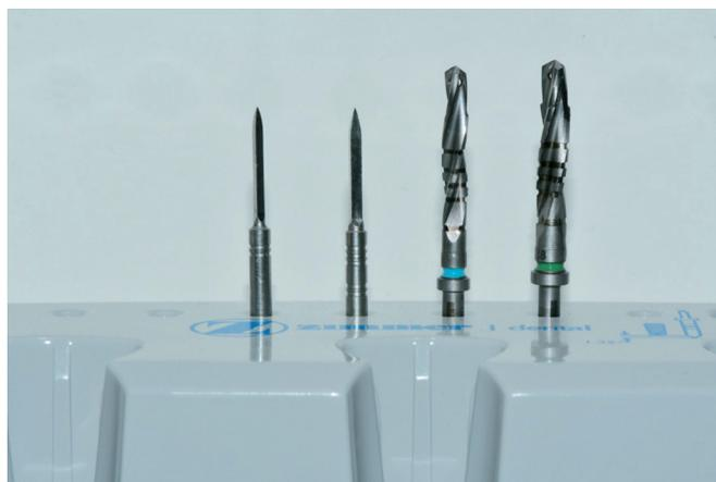
**Figure 11.**—The different milling cutters used throughout the study and their increasing diameter (1.1 mm; 1.9 mm; 2.3 mm; 2.8 mm).
