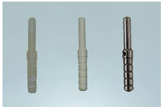
**Figure 9.**—At the beginning of this research the authors reproduced the steel pins produced by Zimmer Biomet using a fiberglass and composite resin material. This pin had a double diameter of 2.3 and 2.8 mm, as the original one.
